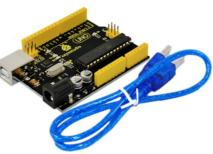
Keyestudio UNO R3 development board is a microcontroller board based on the ATmega328P (datasheet), fully compatible with ARDUINO UNO REV3. It contains everything needed to support the microcontroller; simply connect it to a computer with a USB cable or power it with a AC-to-DC adapter or battery to get started.
