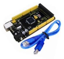
Keyestudio Mega 2560 R3 is a microcontroller board based on the ATMEGA2560-16AU, fully compatible with ARDUINO MEGA 2560 REV3. It contains everything needed to support the microcontroller. With its bootloader, program can be downloaded directly with USB and you don't need to use other external programmer.
